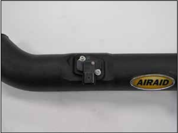
14. Remove the mass air sensor from the factory air filter housing and then install it into the AIRAID intake tube and secure with the provided hardware.
