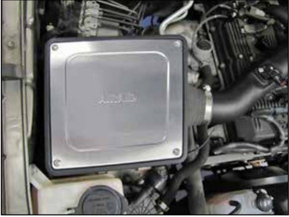
21. Install the provided gasket onto the air filter housing lid and then install the lid onto the air filter housing and secure with the provided hardware.
