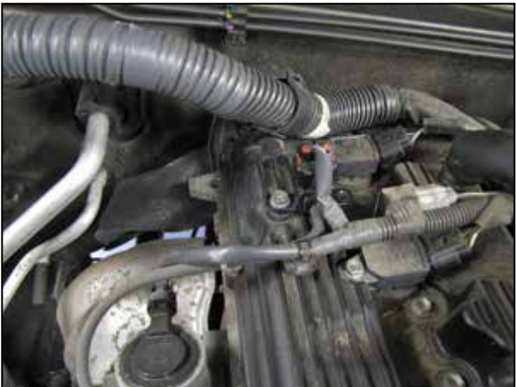
8. Secure the vacuum switching valve to the valve cover using one of the factory plenum bolts.
