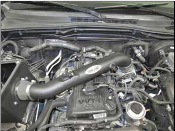
17. Install the AIRAID intake tube into the coupler at the filter adapter and then into the coupler at the throttle body, adjust the tube for best fit and then secure with the provided hose clamps.
