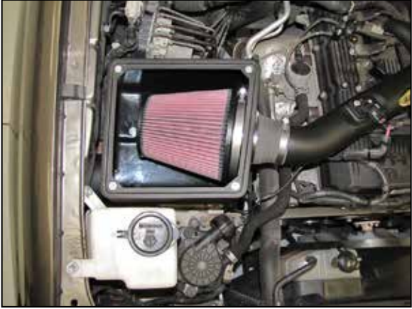
20. Install the AIRAID air filter onto the filter adapter and secure with the provided hose clamp.
