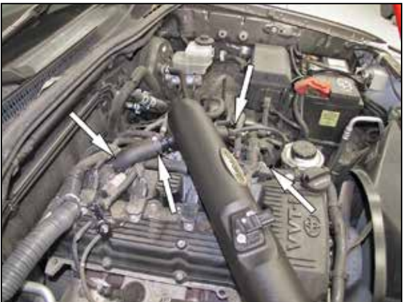
18. Using the provided hose clamps, install the factory crank case vent hose onto the valve cover and vent installed into the AIRAID intake tube. Install the provided vent line onto the fuel pressure regulator and vent installed into the AIRAID intake tube.
