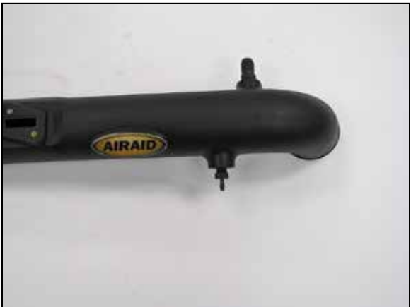
13. Install the provided vent fittings and AIRAID decal onto the AIRAID intake tube as shown. NOTE: Plastic NPT fittings are easy to cross thread. Install the vent fitting “hand” tight, then turn it two complete turns with a wrench.
