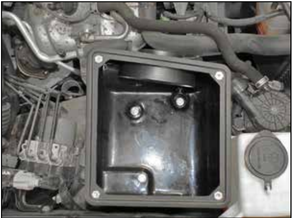
12. Install AIRAID air filter housing into the vehicle and secure with the provided hardware.
