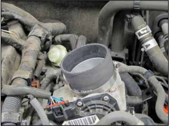
15. Install the coupler hose (084036) onto the throttle body and secure with the provided hose clamp.
