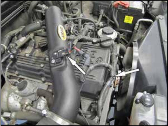
19. Connect the mass air sensor electrical connection and secure the wiring harness with the provided tie wrap.
