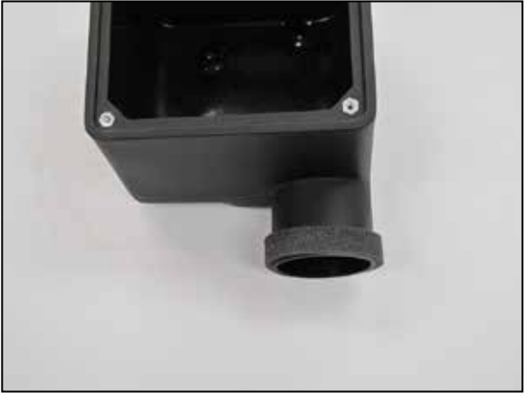
11. Install the foam seal around the AIRAID air filter housing inlet as shown.
