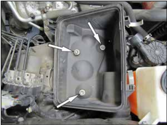
7. Remove the three bolts that secure the lower air filter housing to the inner fender. NOTE: Airaid recommends that customers do not discard factory air intake.
