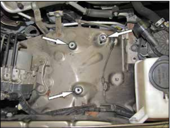
9. Install the provided rubber mounted studs into the inner fender air filter housing mounting locations.
