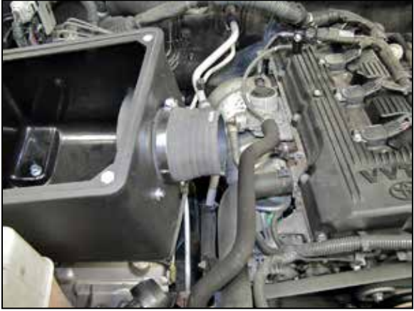
16. Install the coupler hose (084055) onto the filter adapter and secure with the provided hose clamp.
